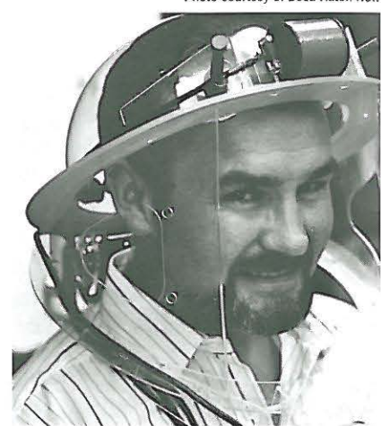
Scott Kelso wearing helmet designed to provide visual feedback of speaker's vocal track events.
