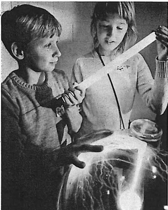
The popular lightning globe demonstrates how the human body conducts electricity that can light a fluorescent bulb.
